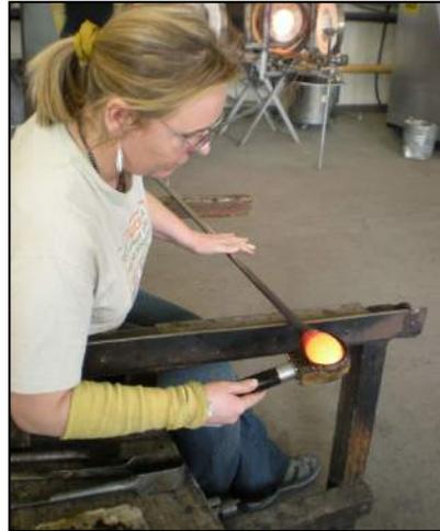
More glass is gathered over this and the bubble is blown bigger and bigger with the glass blower shaping it into a large cylinder. During this process the glass is reheated when it cools too much.
