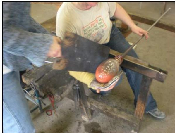
After two further gathers of glass the bubble is being shaped with wet paper. An assistant shields the glass-blower from the heat with a wooden paddle.
